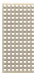
136 pin BGA (0.4 mm pitch)
