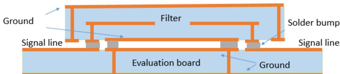
Fig.5 Side view of filter
