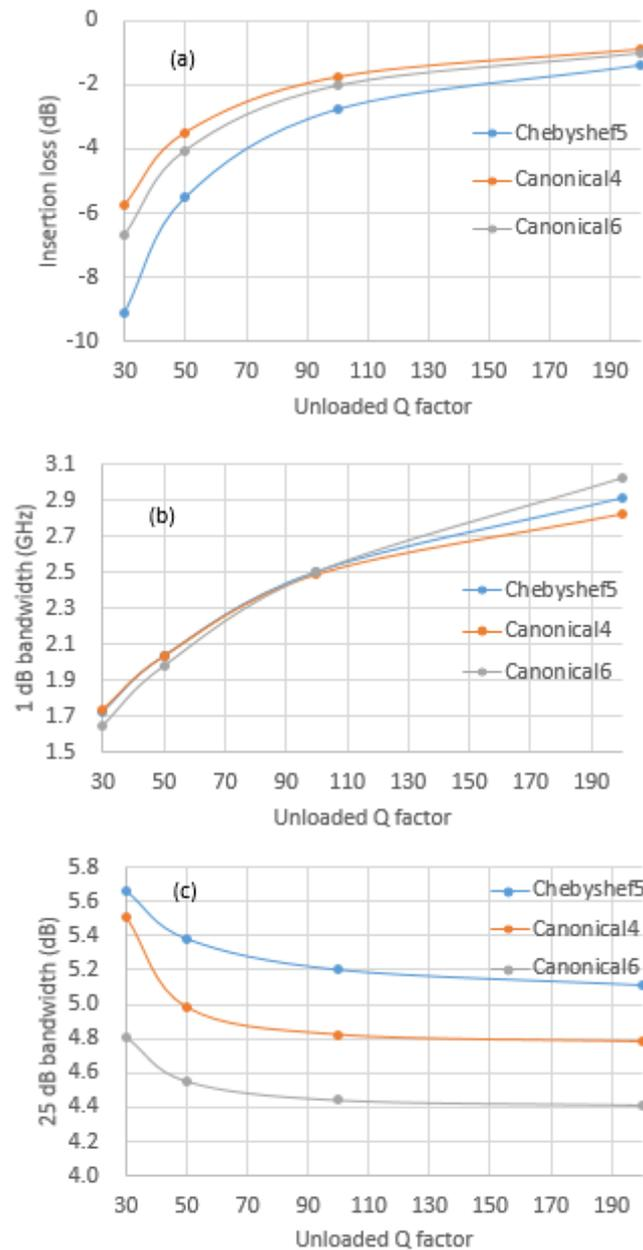
Fig.4 Unloaded Q factor dependence of (a) peak of passband, (b) 1 dB bandwidth, (c) 25 dB bandwidth.
