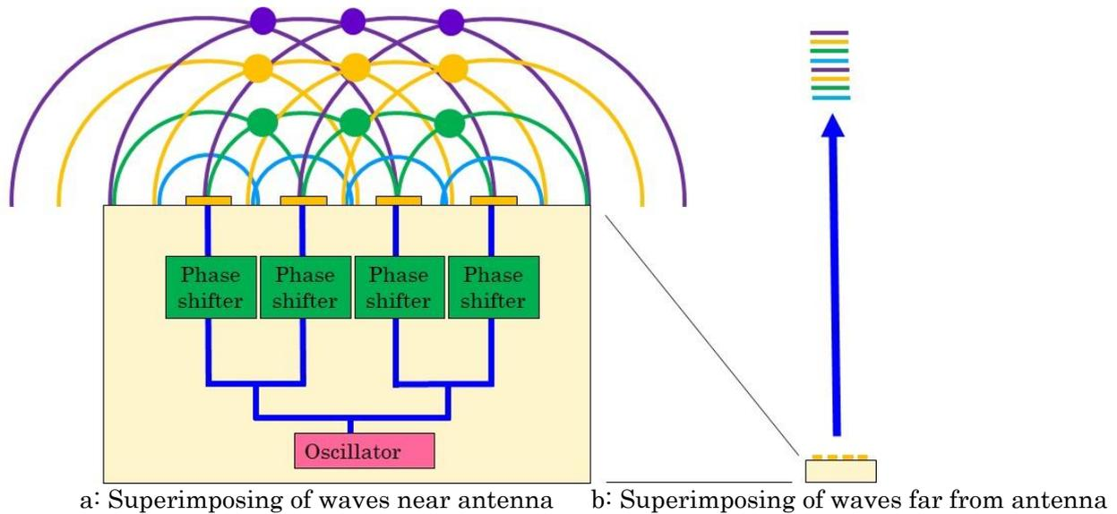
Fig. 6 Spread of waves from antenna element and their superimposing
