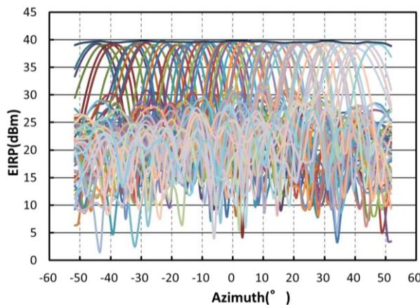
Fig. 9 Example of beamforming (graph of beam profile)
