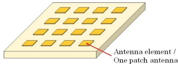
Fig. 2 Configuration of phased array antenna
