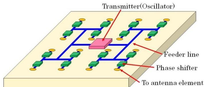
Fig. 3 Schematic diagram of driving circuit of phased array antenna
