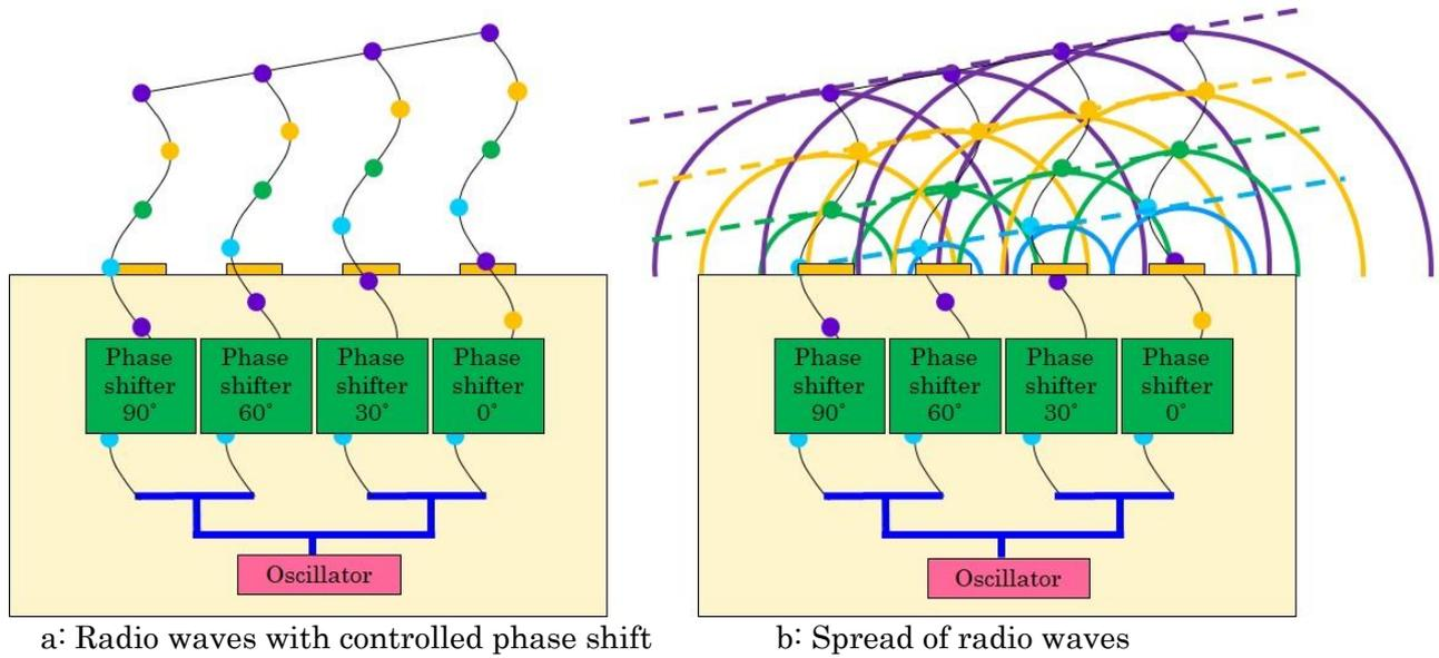
Fig. 8 Propagation of radiated radio waves with controlled phase shift
