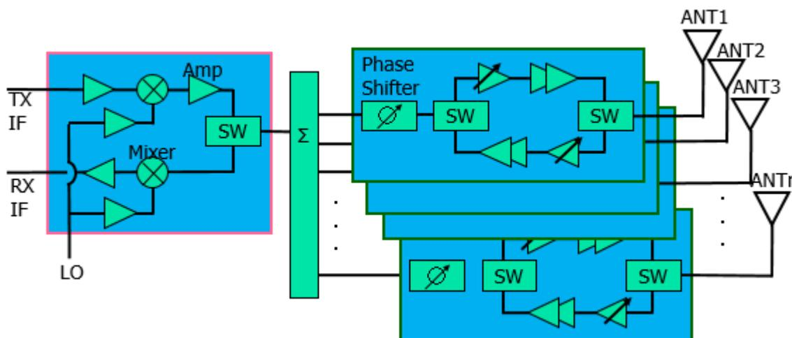
Fig. 1 Block diagram of RF module with phased array antenna
