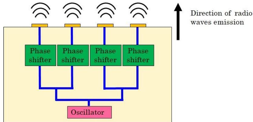
Fig. 4 Schematic diagram of phased array antenna consisting of four elements
