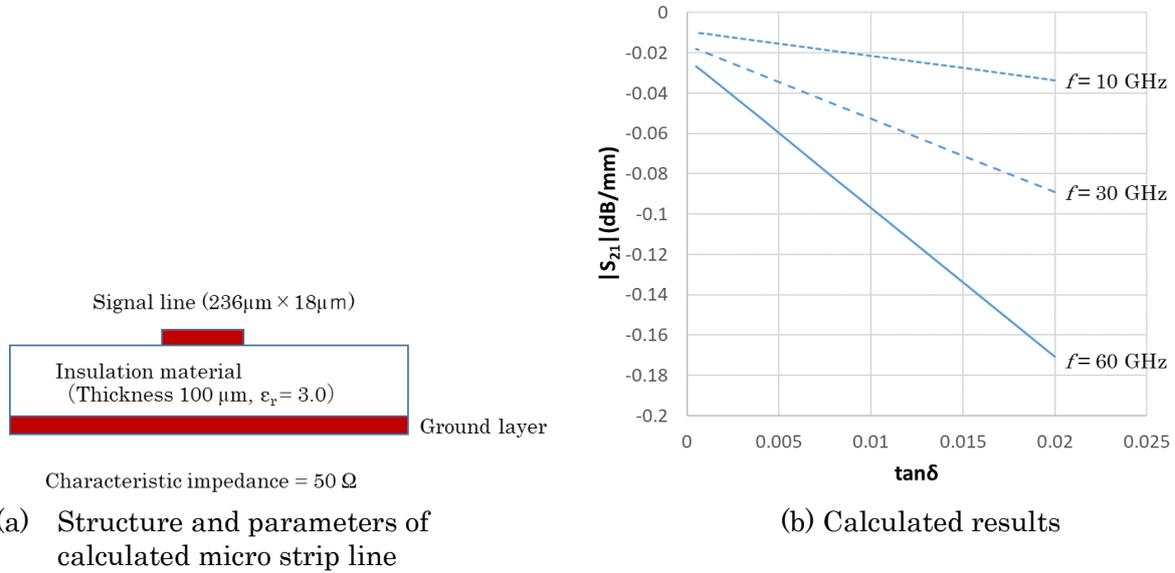
Fig. 2 Relationship between transmittance, transmission frequency and  $\tan \delta$ .
