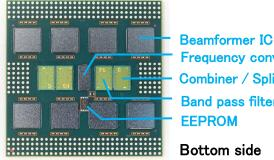
Frequency conversion IC Combiner / Splitter Band pass filter
